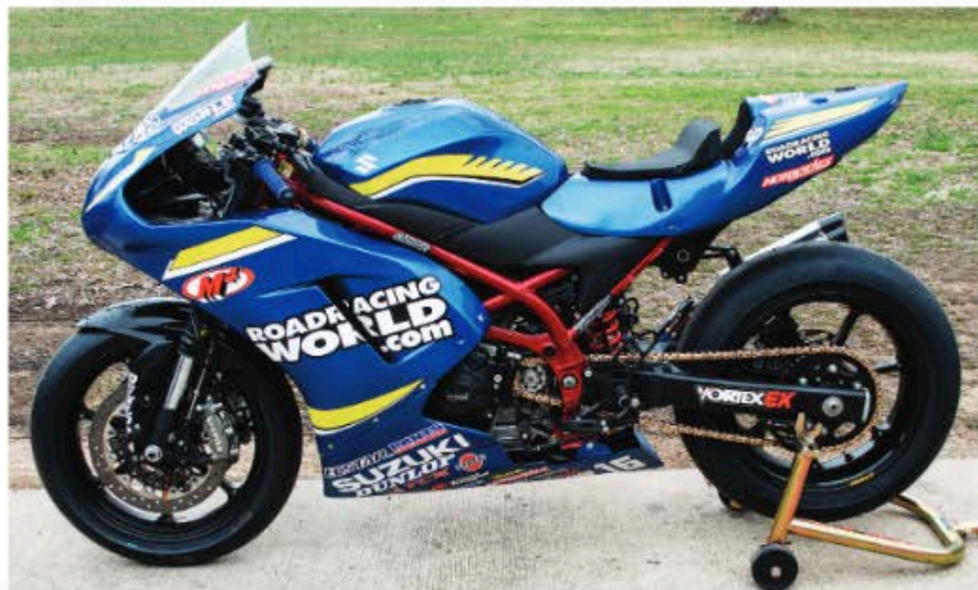
(Top) Twins Cup Champion Alex Dumas on the project racebike. Photo by Brian J. Nelson. (Above & Below) The SV650 with and without bodywork. Features include GSX-R600 forks and brakes; Dymag wheels; Hotbodies GSX-RR replica bodywork; carbon-fiber airbox; GBRacing covers; K-Tech shock; Vortex clip-ons and sprockets; Woodcraft rearsets; and a lot more we'll cover later. Photos by John Ulrich.
