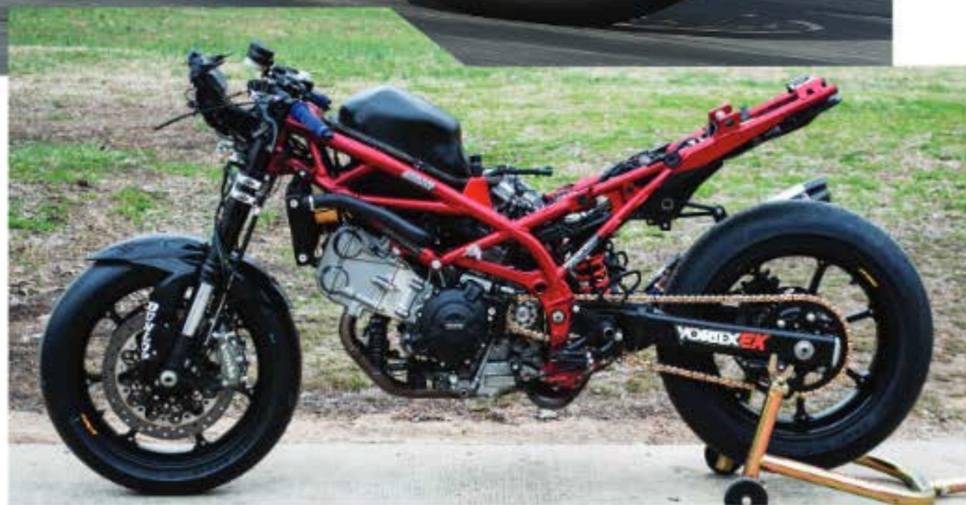
(Top) Twins Cup Champion Alex Dumas on the project racebike. Photo by Brian J. Nelson. (Above & Below) The SV650 with and without bodywork. Features include GSX-R600 forks and brakes; Dymag wheels; Hotbodies GSX-RR replica bodywork; carbon-fiber airbox; GBRacing covers; K-Tech shock; Vortex clip-ons and sprockets; Woodcraft rearsets; and a lot more we'll cover later. Photos by John Ulrich.
